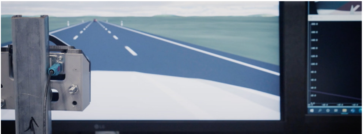
Hardware-in-the-loop: A HIL bench presents simulated inputs to real hardware.
